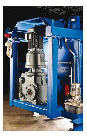
Automatic mechanical bag opening is the first step of a process which is carried out in a modern waste management plant. Equipment offered by CONTROL PROCESS are designed to open and emptying plastic bags filled with all kinds of waste and recyclable materials.
